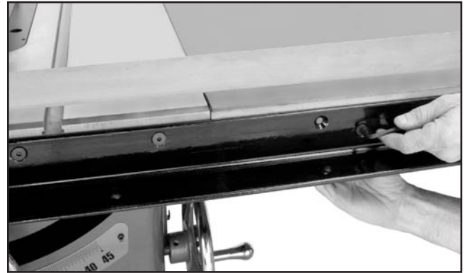
Figure 15. Aligning main extension table.
